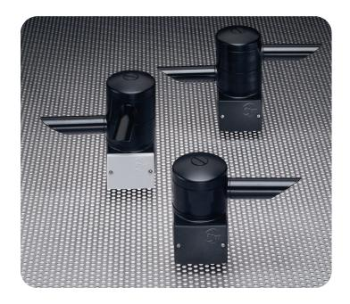
The Opticom 700 Series Detectors transform the optical energy detected from an approaching, vehicle–mounted Opticom Emitter to an electrical signal. The electrical signal is transmitted along a cable to the Opticom Phase Selector or Opticom Discriminator for processing.
