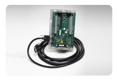
Opticom 768 Auxiliary Interface Panel (AIP) provides a convenient method to interconnect Opticom 762 and 764 Phase Selectors with terminals inside a traffic cabinet. The 768 AIP is designed specifically for use with the Opticom 762 and 764 phase selectors. It is not intended to be used with other phase selectors.
